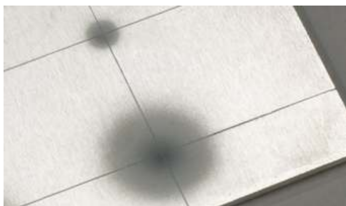
Pin-point accurate and cost-effective sandblasting. Above: Renfert focused jet, below: focused jet of a competitor
