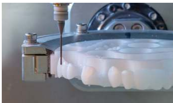
Optimum suction of the chips during milling
